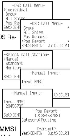
7. When finished entering the MMSI number, press and hold the **[CALL(ENT)MENU]** key.
