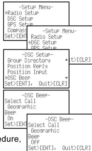
To enable the ringer tone, repeat the above procedure, press the [**▲**] key to select "On" in step "6" above.
