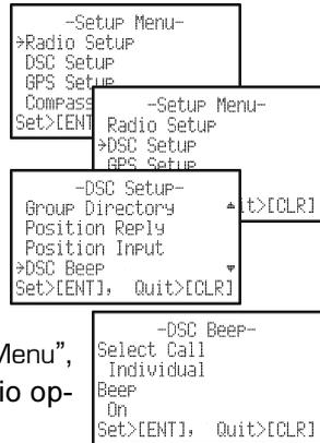
To enable the ringer tone, repeat the above procedure, press the [▲] key to select "On" in step "6" above.
