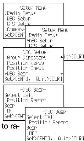
To return to enabling the ringer tone, repeat the above procedure, press the [▲] key to select “On” in step “5” above.
