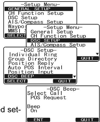
To re-enable the ringer tone, repeat the above procedure, rotating the **CHANNEL** knob to select “On” in step “5” above.
