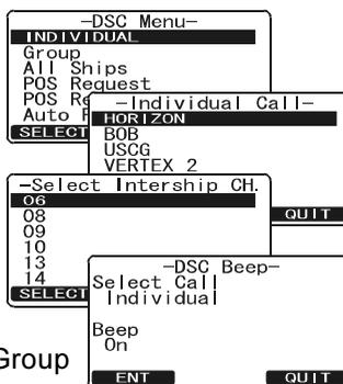
To re-enable the ringer tone, repeat the above procedure, rotating the CHANNEL knob to select “On” in step “6” above.
