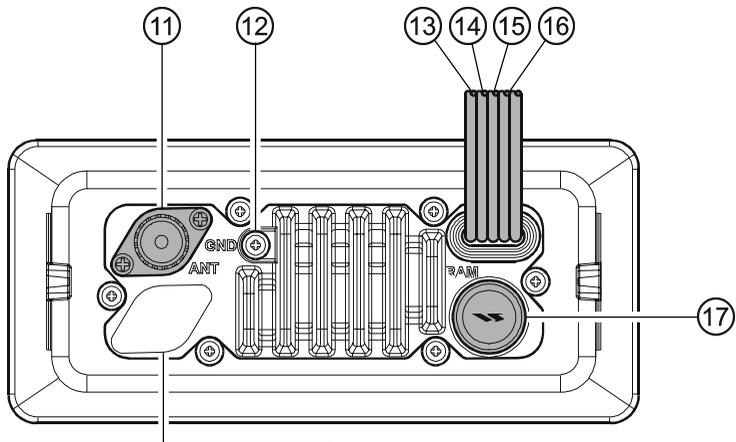
**Never remove this rubber cap. When this rubber cap is removed, the water resistance performance is lost.**
