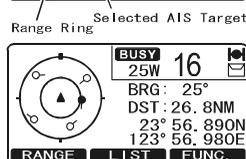
3. Rotate the **CHANNEL** knob to select the MMSI number (or vessel name). The selected AIS target is displayed with “●” icon, other station is displayed with “○” icon.
