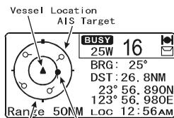
2. Press the one of the soft keys momentarily, then press the **[LIST]** soft key to show a list of AIS vessels being received.
