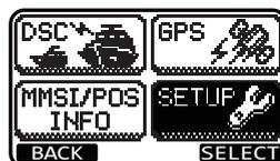
4. Select “UNIT OF MEASURE” with the **▲ / ▼** keys, then press the **SELECT** soft key.
