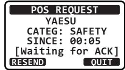
8. When the **GX1300E** receives the position from the polled vessel, the **GX1300E** will produce a ringing alarm sound and the position from the polled vessel is sent to a GPS chart plotter via NMEA 0183. (DSC BEEP needs to be enabled to hear alarm.)
