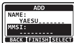
11. Select "MMSI" with the ▲ / ▼ keys, then press the **SELECT** soft key.
