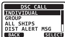
5. Press the **▲ / ▼** keys to select an individual you want to contact, then press the **SELECT** soft key.
