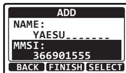
16. Press the **FINISH** soft key to save the entered address.
